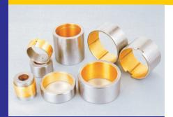
UF-850 is a steel-bronze bearing, which is sintered with 6-6-3 bronze in its inside as a lining and uses 20# steel as backing. The performance of this structure parallels that of all 6-6-3 bronze bearing but saving cost. So it can replace thick wall bronze bearing and improve product competence to use in oil box, construction machines and other high precision but low speed occasions.
