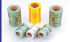
FD-Al linear motion bearing is one kind of self-lubricated linear motion products. They're used in moulds' slipways and precision machines instead of steel rolling bushings. The bearings have obvious advantages such as low noise, low cost and working without oil.
