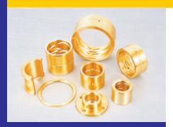
JDB-1 U takes oil in inner grooves to work. It can be used in low speed because of larger load, longer life and higher HB than Al-Cu bearing. Now JDB-1 U is mostly used in gear cases and joint parts of grabs.
