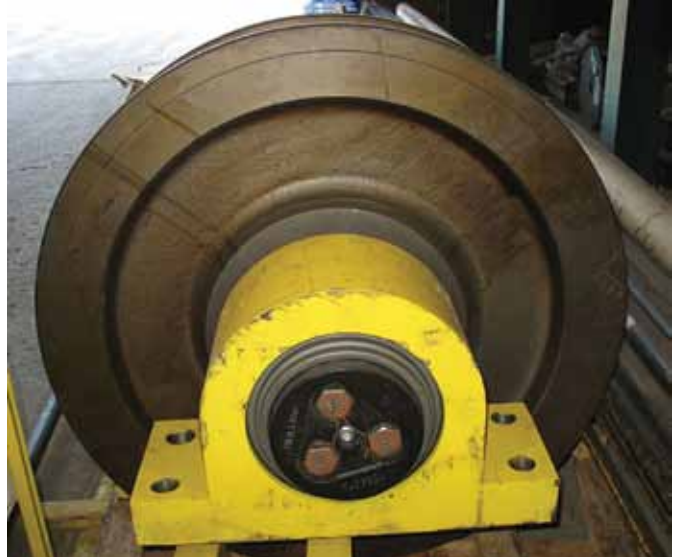
Fig. 12 AP bearings used in pillow block application
