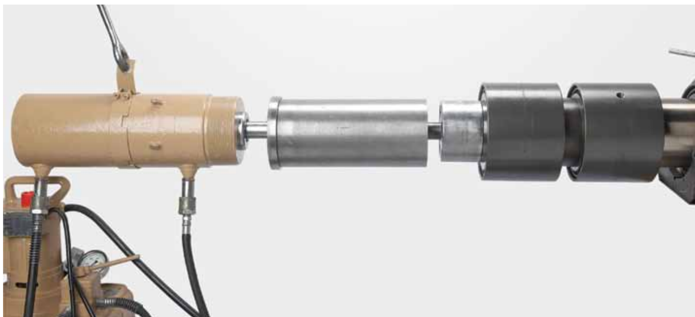
Fig. 28 Tooling used to push bearing onto shaft
