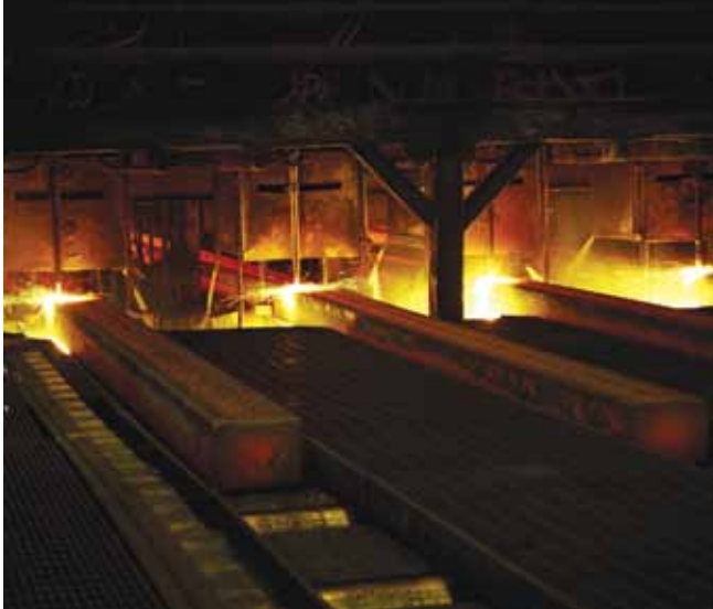
Fig. 11 AP bearing equipped runout tables
