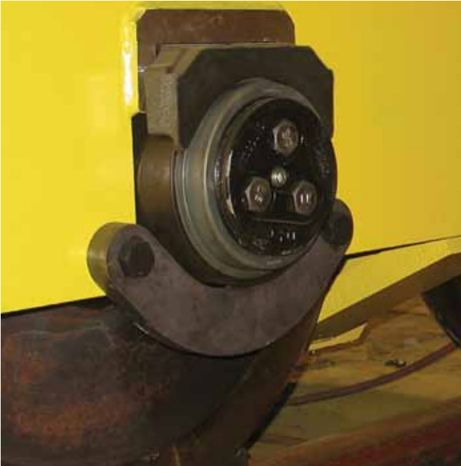
Fig. 8 Narrow adapter mounting on trolley safety bar
