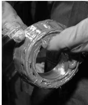
Fig. 23. Grease can easily be packed by hand.
