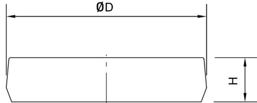
**Table 2.40 Dimensions of Bolt Caps for Rail Mounting Holes**
