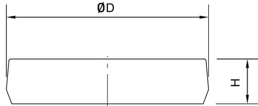
**Table 2.66 Dimensions of Bolt Caps for Rail Mounting Holes**
