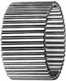
In certain applications, the limited amount of space available for bearings and the loads to be supported require the use of a full complement of needles independent of any system of retention. The length of the needle is determined in relation to the load capacity required.
