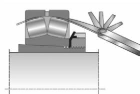
The clearance can be measured by sliding a feeler gauge between the outer ring and the rollers. For large bearings do not use feeler gauges over 0.150 mm thick since they are too stiff to take the shape of the outer ring raceway. Instead of thick gauge use a combination of thin gauges by stacking them up for measurement.
