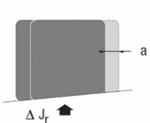
The residual clearance of the bearing must be checked after fitting. This check is vital for bearings with a tapered bore. Relation between the axial displacement 'a' of a tapered bore bearing and the corresponding reduction in its radial clearance,  $\Delta Jr$ :
